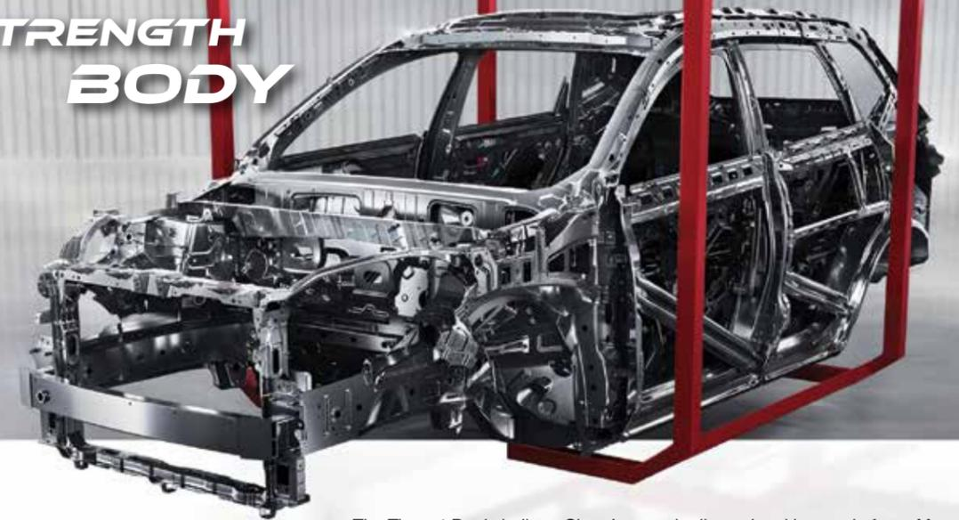
The Tiggo 4 Pro is built on Chery's new six-dimensional beam platform. More than two-thirds of the vehicle's frame and structure is built with high- and ultra-high strength steel, and the 6-dimensional design gives it unmatched torsional rigidity and crash safety.
